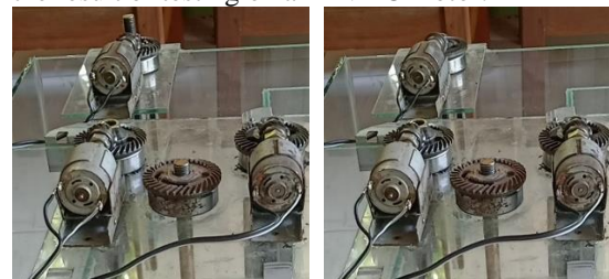
(a). 12V DC motor when opening door 1
